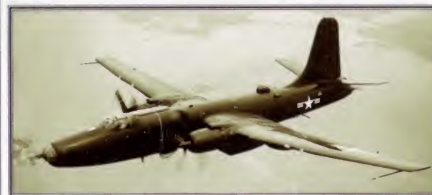
◀ First production Mercator The first production P4M-1 early on in its career; the main undercarriage did not retract fully into the Mercator's wing and was surrounded by a fairing on the lower wing surface.
